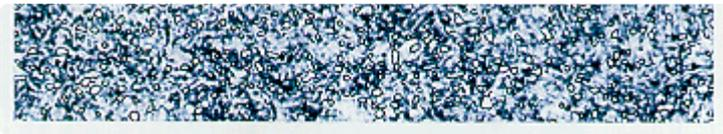
Optimized hardening conditions give optimal austenite content (15%), many uniformly distributed carbides.
