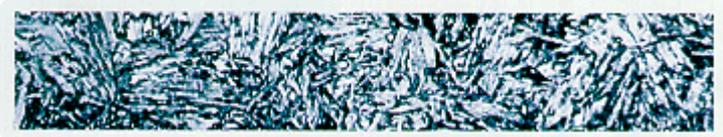
Too high hardening temperature gives coarse structure, high austenite content (30%), few carbides.
