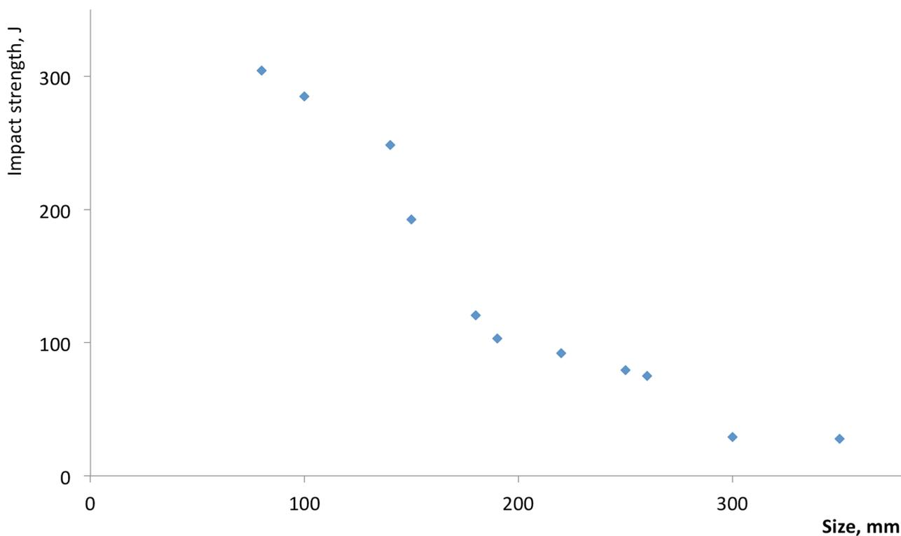
Figure 2. Typical impact energy values for SAF™ 32760 in different sizes at -46°C (-50°F), using standard Charpy V specimens.
