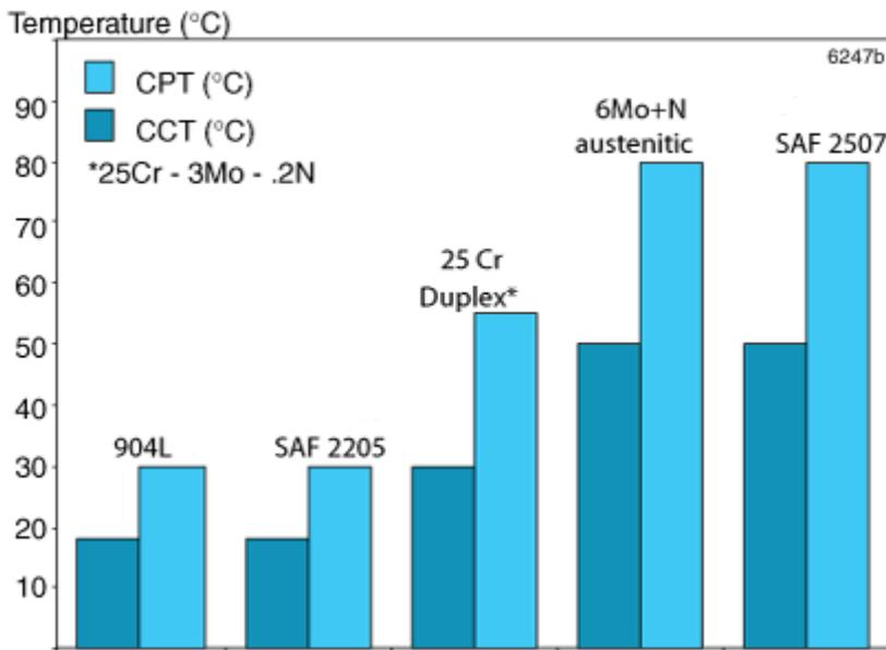
Figure 4. Critical pitting and crevice temperatures in 6% FeCl<sub>3</sub>, 24h (similar to ASTM G48).
