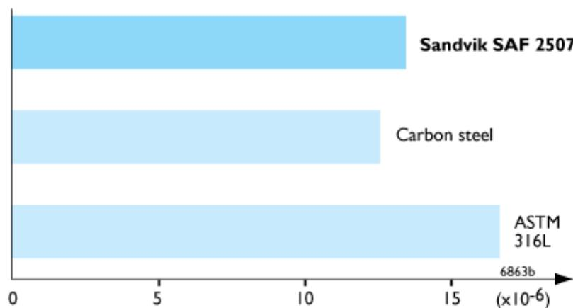
Figure 3. Thermal expansion, per  $^{\circ}\text{C}$  (30-100 $^{\circ}\text{C}$ , 86-210 $^{\circ}\text{F}$ ).
