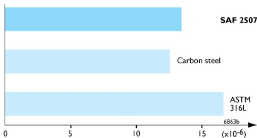
Figure 4. Thermal expansion, per °C (30-100°C, 86-210°F).
