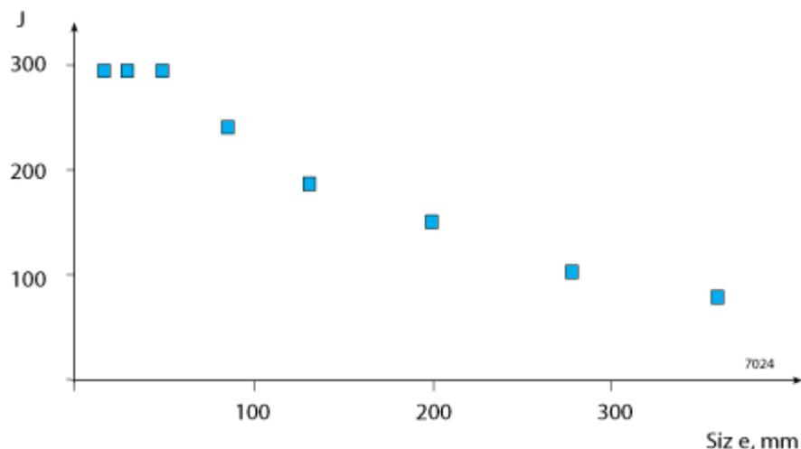
Figure 3. Typical impact energy values at -20° C (-4°F), for SAF 2507 bar steel.
